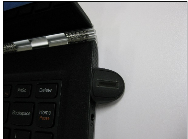
Figure 7: AuthenTec Eikon Mini USB Fingerprint Reader plugged into the author's Lenovo Yoga 900
